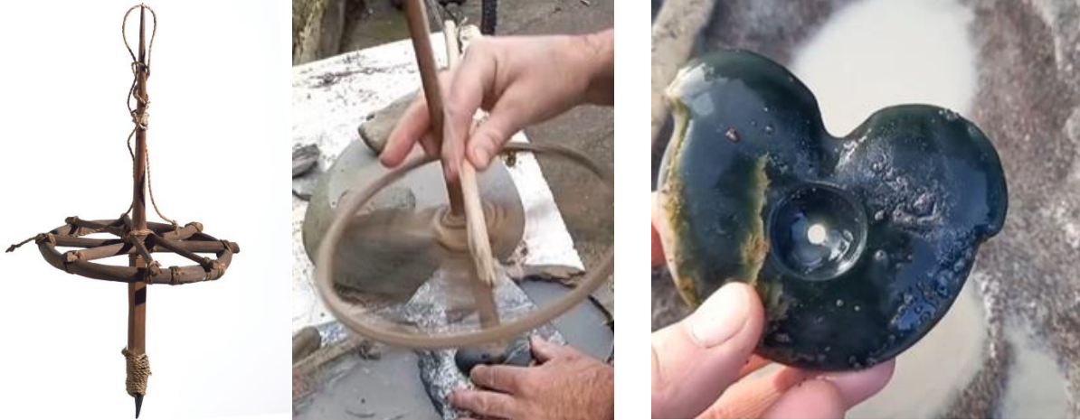
A pirori (cord drill), used by Māori to create holes in weapons, adornments, etcetera. xiv
