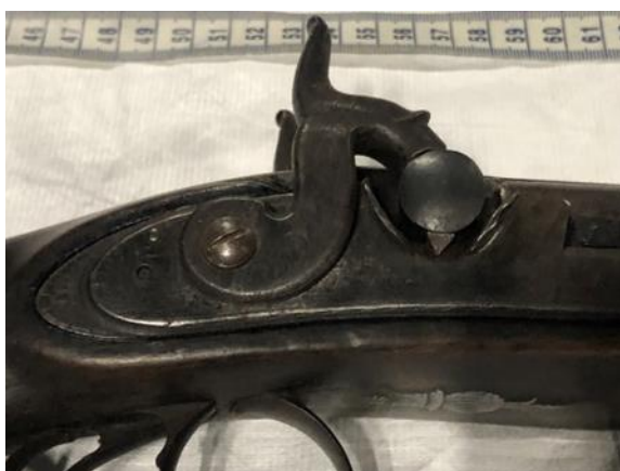
Figures 21 & 22: The righthand side lock plate, the flintlock cock has been replaced with a hammer, percussion cap and nipple (left image). Work done where the pan and frizzen would have been (right image).
